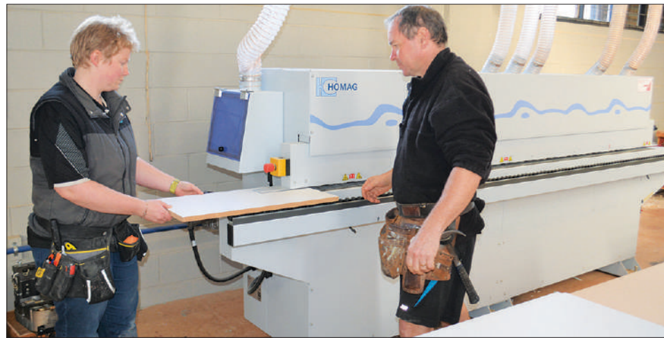
Emma Clark and Shaun McDowell using their new Homag edge bander, to apply a laser edge to what will become part of someone's new kitchen.
