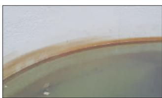
Manganese buildup on tanks - this is what happens on the inside of water pipes.
